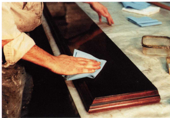
Photo 1a & b — Finish can be spread from center toward edges with a soft-bristled brush (a). Later, wipe off unset finish (b).
