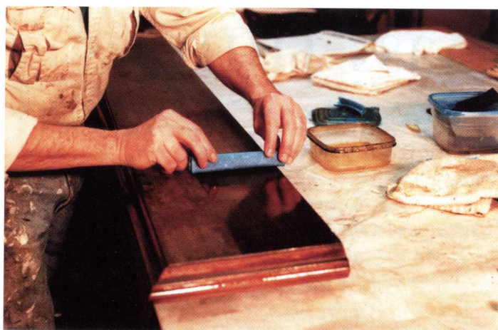
Photo 10 — Use “pad” to apply finish, beginning a few inches from edge.
