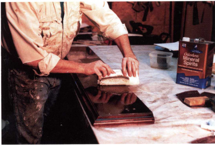
Photo 3 — Wipe off old finish residue with clean terry cloth shop towel.
