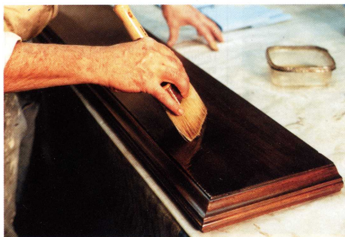
Photo 1a & b — Finish can be spread from center toward edges with a soft-bristled brush (a). Later, wipe off unset finish (b).
