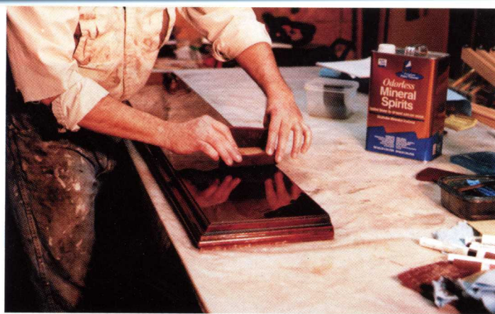
Photo 2 — Scrub the surface to be cleaned with mineral spirits using 3M maroon finishing pad.
